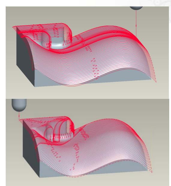
Defined cut feed: 1000mm/Min. X motor has to run at 1000mm/min, Y motor does nothing.
