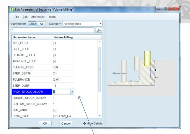
Add 1mm to these 3 boxes. If you are working on the routers, there is no need to program the spindle speed, it's done manually.
