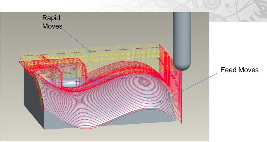
Playing the path shows us the machining cycle. You can see that there is a lot of rapid moves, almost as many as feed moves (in red). This is not an efficient machining cycle.
