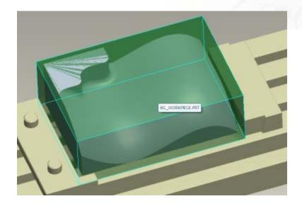
This part is aligned to the top of the workpiece, this means the top of the block will not be machined and our block will remain at 55 thick. Our part is placed in from the edges by 5mm to allow machining all round.
