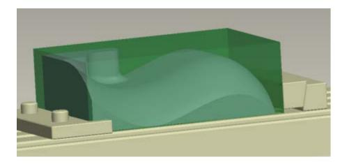
This part is aligned to the bottom of the block, we will need to remove material from the top using a volume rough and our block will finish at 50mm, as before, the part is inset by 5mm in X&Y to allow machining all round.
