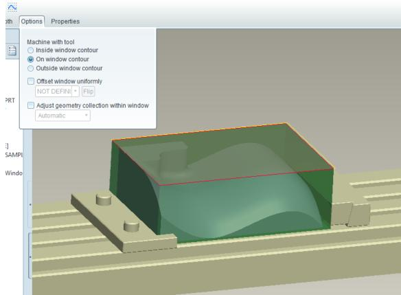
window contour. I.E. it will machine past the window to the centre line of the cutter.
