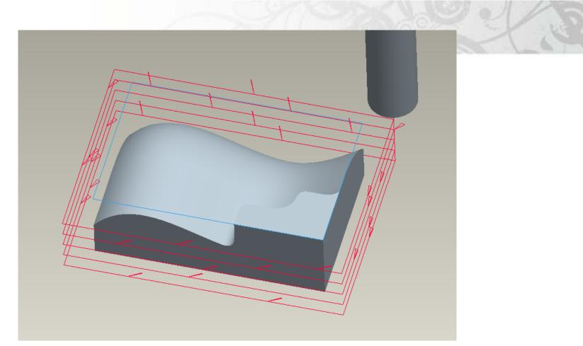
Using a trajectory mill cycle allows us to machine the straight sides, it's also faster. Don't forget to set the stock allow back to 0 in the parameters! It makes sense to use the same tool that we used for roughing to save on tool changes, you could also finish the top flat surface but we're going to profile mill that at the same time as the contour to ensure dimensional accuracy.
