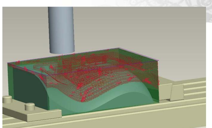
Playing the path shows us that the cutter satisfactorily roughs out our part. Note that the outside has not been machined in this instance and there is 1mm left on the top surface that needs to be removed. The display shows us the centre line movement of the cutter only with rapid moves being shown as a yellow dotted line. We can see that the cutter spends all of it's time machining and very little time making rapid moves, this shows that an efficient cutting process has been defined.
