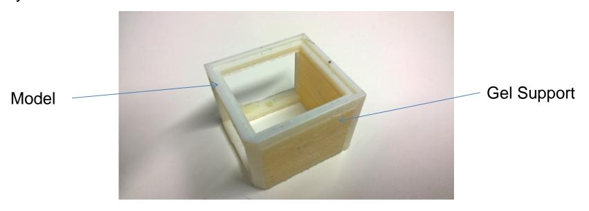
If your part is reasonably strong, it is quite easy to remove the support by using the water blast cabinet. If you are worried about breaking your part then you can pick off the largest parts and use a brush to remove the remainder. Leaving your part in water for a few hours will soften the support before removal. Any residue can be removed in a 10% caustic soda solution.
