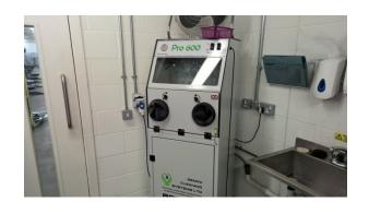
The water blast cabinet is situated in LDS.0.07 (the CNC workshop). It should only be used to remove support, it is not for cleaning parts!
