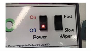
Make sure the power is set to on at the rocker switch located on the front panel.
