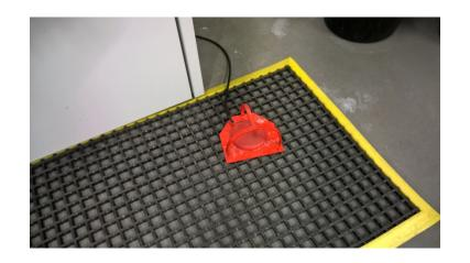
To operate the machine, there is a foot switch, simply press to actuate the water. If you are using the flexible line, make sure you have hold of it before you press the foot pedal. Pass your part under the jet and it should push off the support. If your part is delicate then hold it further away from the nozzle or reduce the pressure using the blue adjustment Knob.
