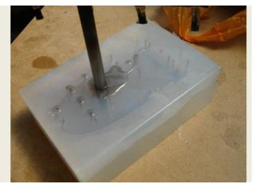
Different resins require different operating temperatures for the resin and the mould. You must refer to the material data sheet for the chosen resin to ensure the correct operating temperatures, mixing ratios and venting times are used.
