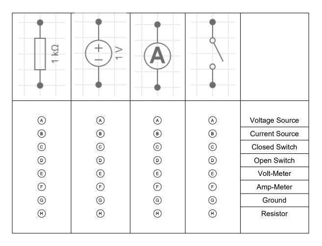
b) For the same four elements, assume they are used as part of a circuit. Can the voltage across the element be positive, zero, or negative (negative pole at the top)? Several correct answers may apply to each element.
