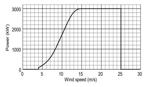
d) Combination of the whole of the Weibull distribution with the whole of the turbine power curve provides a first estimate of electricity yield.
