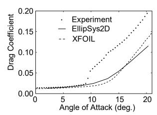
$$C_{\rm d} = \frac{drag}{\frac{1}{2}\rho U^2 A} = \frac{drag / unit \, span}{\frac{1}{2}\rho U^2 c}$$
