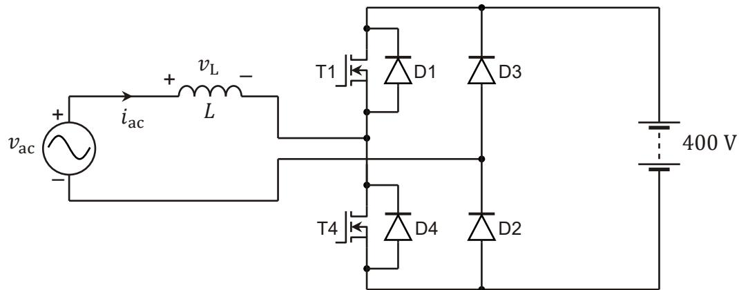
The transistors, T1 and T4, are switched alternately at high frequency
