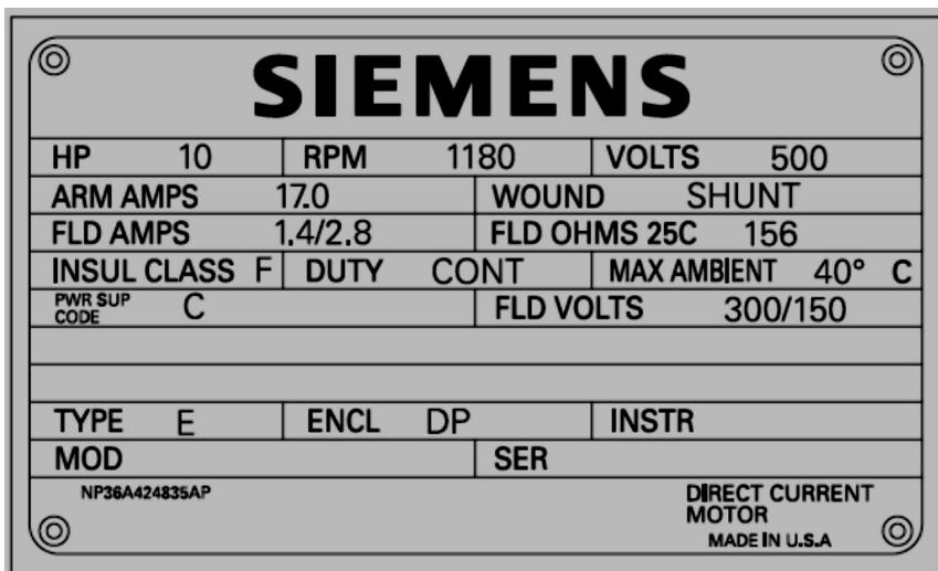
The motor armature has negligible resistance and 20 mH inductance. The chopper is supplied from a constant DC bus voltage of 500 V and switched at 20 kHz. It is required to operate the motor at its rated torque and  $2/3$  of its rated speed.
