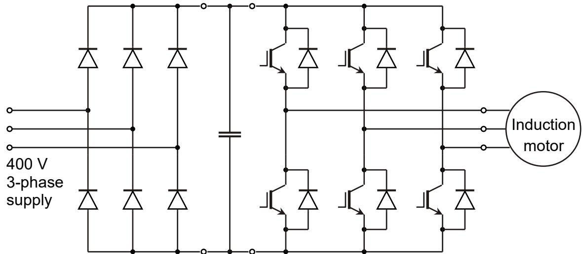
Explain how this circuit can be used to vary the speed of the pump, and describe a simple way to create the switching pattern necessary for the transistors.
