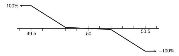
The horizontal axis is frequency in hertz. The vertical axis is active power.
