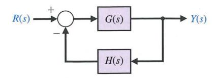
(b) Obtain the closed-loop transfer function for the system shown above, when process transfer function  $G(s) = \frac{225}{s(s+12)}$  and sensor transfer function H(s) = 1.
