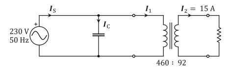
Calculate the required value of capacitance.
