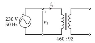
You may assume the transformer is lossless and neglect leakage reactances. But it is *not* completely ideal, because it does have a significant inductive magnetising current.
