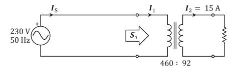
Calculate the complex value of the primary current  $I_1$ , including the magnetising current from part c). You may assume the transformer is lossless and neglect leakage reactances.
