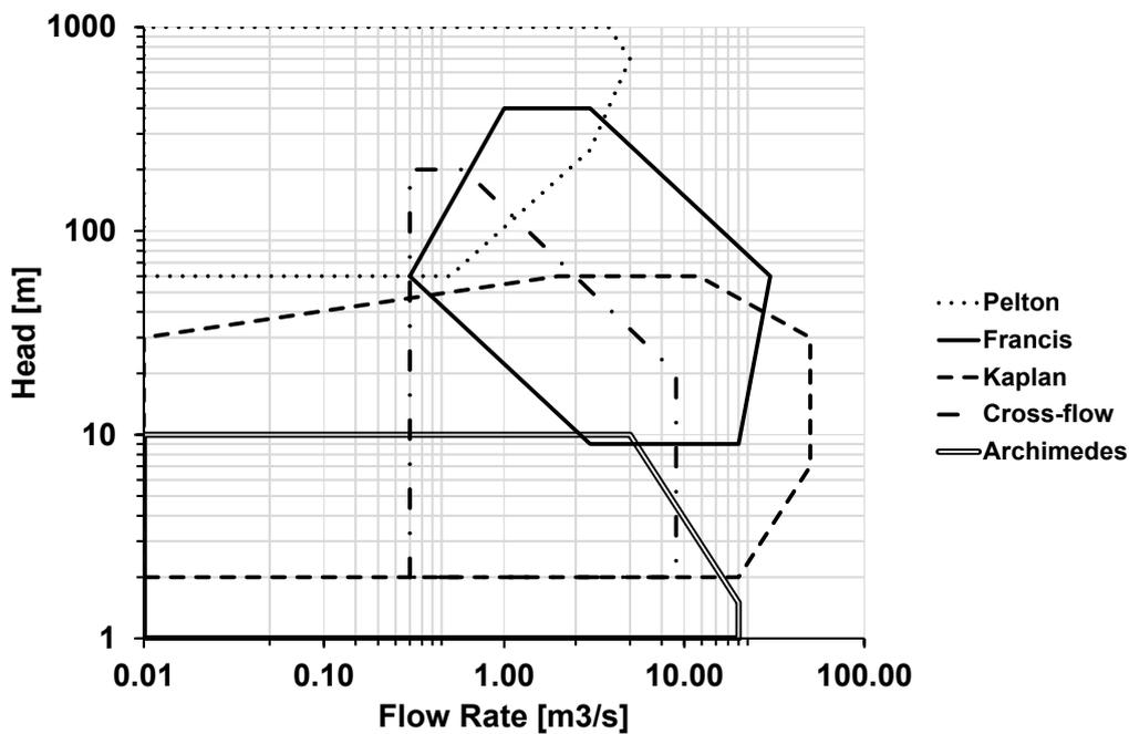
Power output of a hydropower scheme:  $P = \eta\rho gQH$
