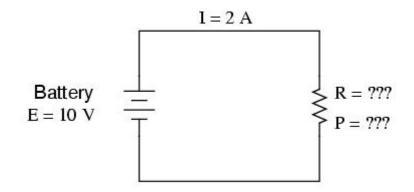
All we've been given here to start with is the battery voltage (10 volts) and the circuit current (2 amps). We don't know the resistor's resistance in ohms or the power dissipated by it in watts. Surveying our array of Ohm's Law equations, we find two equations that give us answers from known quantities of voltage and current:
