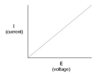
The straight-line plot of current over voltage indicates that resistance is a stable, unchanging value for a wide range of circuit voltages and currents. In an "ideal" situation, this is the case. Resistors, which are manufactured to provide a definite, stable value of resistance, behave very much like the plot of values seen above. A mathematician would call their behaviour "linear."
