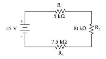
It should be apparent that the voltage drop across each resistor is proportional to its resistance, given that the current is the same through all resistors. For example, the voltage across  $R_2$  is double that of the voltage across  $R_1$ , just as the resistance of  $R_2$  is double that of  $R_1$ .
