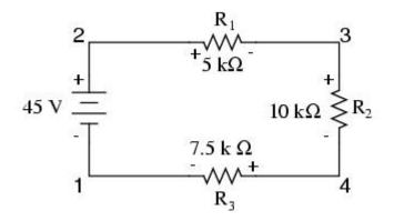
If we were to connect a voltmeter between points 1 and 2, black test lead to point 1 and red test lead to point 2, the meter would read +45 volts. Typically the "+" sign is not shown (but implied) for positive readings in digital meter displays. However, for this lesson the polarity of the voltage reading is very important:
