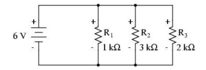
Using Ohm's Law (I=E/R) we can calculate each branch current: Knowing that branch currents add up in parallel circuits to equal the total current, we can arrive at total current by summing 6mA, 2mA, and 3mA:
