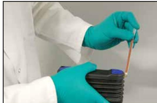
Break off the two ends of the color coded tube. Each pump is generally equipped with a system that allows the tubes to be broken without any risk to the operator or maintenance technician.
