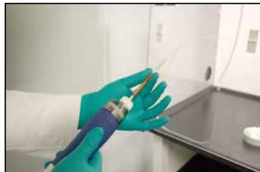
Connect the broken tube to the pump, being careful to verify that the tube is inserted in the correct direction. The color coded tubes are marked with this information.
