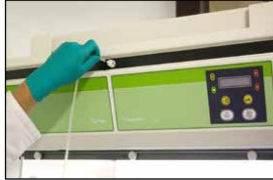
Connect one end of the silicone tube to the sampling port located on the control panel of your Captair<sup>®</sup> Flex<sup>™</sup> fume hood.
