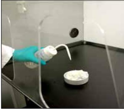
Evaporate a sufficient amount of the chemical for testing purposes within the enclosure. To do this, soak a rolled up piece of cloth in a container placed inside the enclosure of your Captair<sup>®</sup> Flex<sup>™</sup> fume hood.
