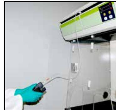
After connecting the flexible silicone tube to the other end of the broken tube, collect an air sample using the pump. Refer to the instructions provided with the tubes for the number of times to pump.
