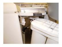
Insert the Pretreatment (PT8 or PT16) in the left hand retaining block pushing it home until it clicks into position and retaining mechanism clicks up.
