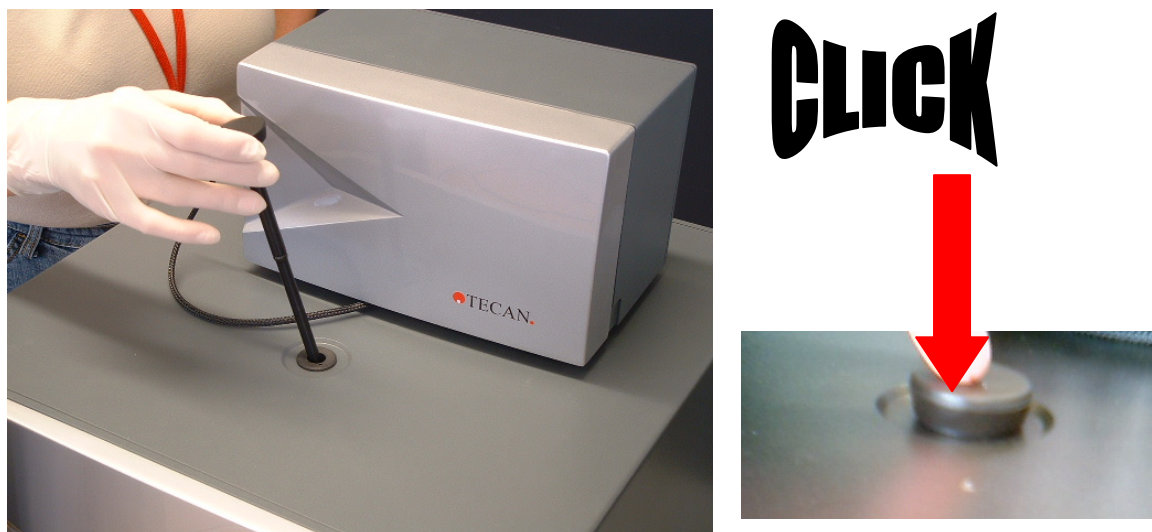
Picture 2-1: Inserting the injector carrier into the injector port
