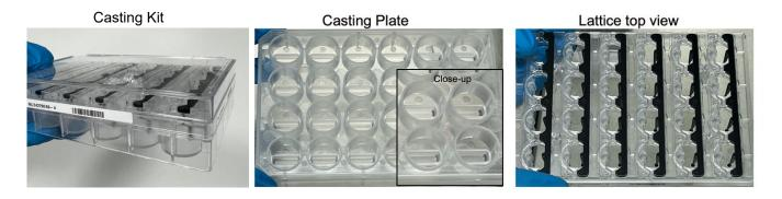
b. Casting Plate and Lattice is used together to cast 3D engineered muscle tissues.
