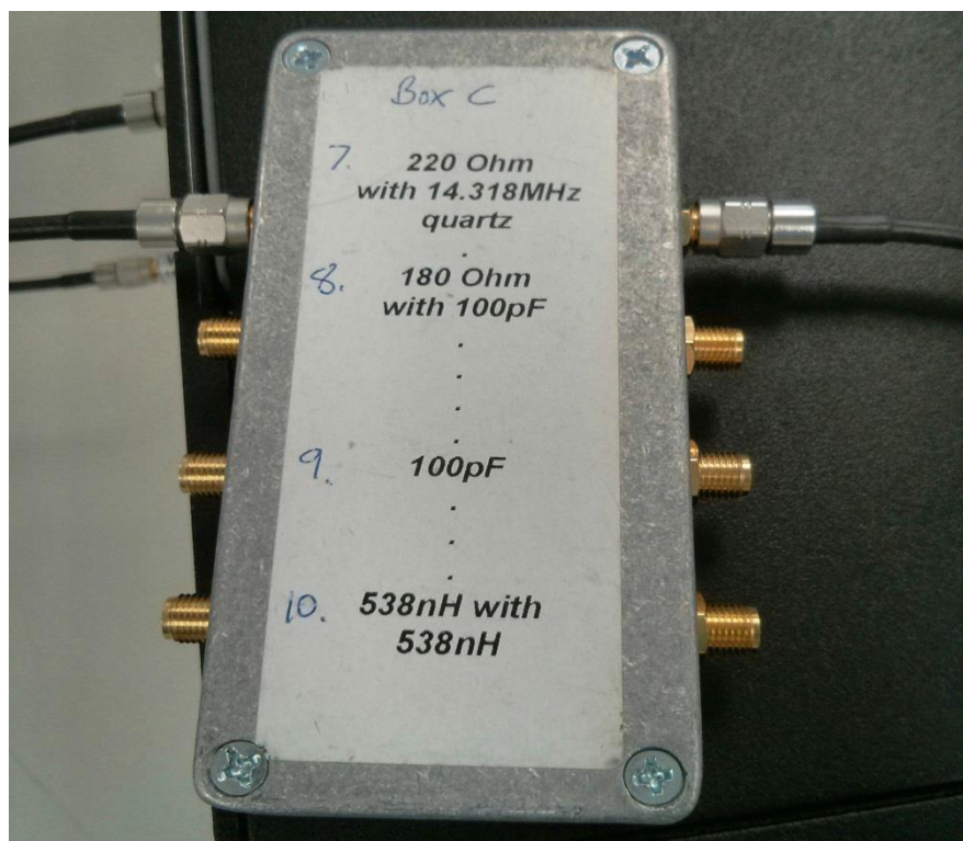
Figure 28: Snapshot of SensAND instrument connected to 14.318 MHz quartz circuit along with 220 ohm resistor
