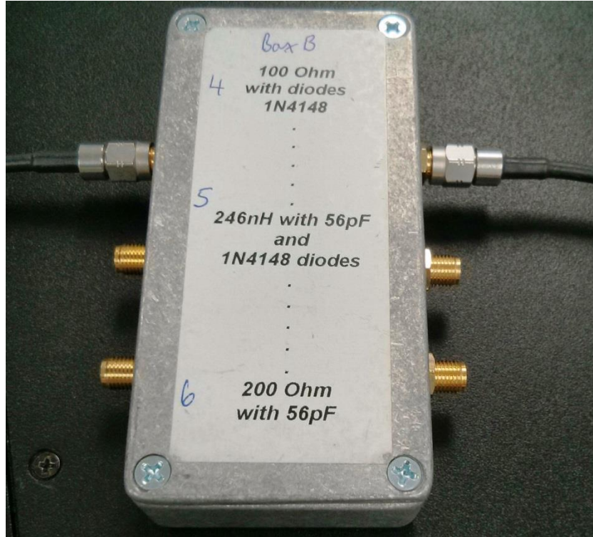
Figure 31: Snapshot of SensAND instrument connected to a circuit comprising of diodes and 100 ohm resistor
