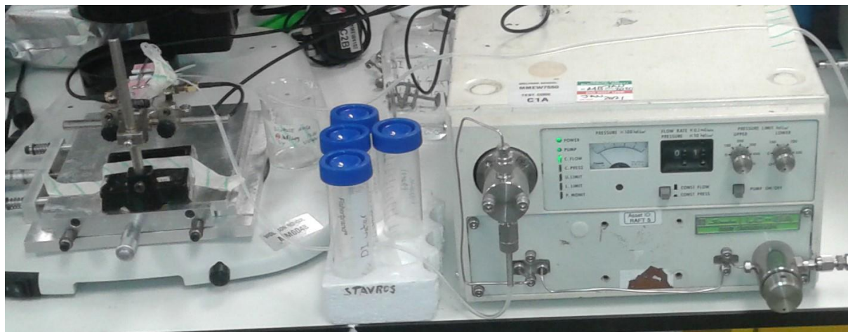
Figure 5. Picture of HPLC pump connected to the microfluidic cartridge. An HPLC pump is to be used in conjunction with peristaltic pump (not shown).
