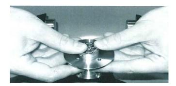
**NOTE:** When using Aerosol tight rotor lids the rotor can only be removed with the lid closed. This is to protect the user and the samples.
