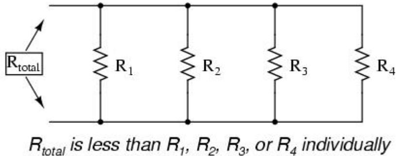
Total parallel conductance is *greater* than any of the individual branch conductances because parallel resistors conduct better together than they would separately:
