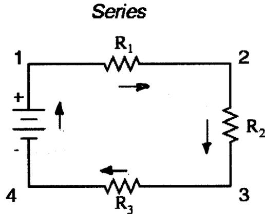
Here, we have three resistors (labelled  $R_1$ ,  $R_2$ , and  $R_3$ ), connected in a long chain from one terminal of the battery to the other. (It should be noted that the subscript labelling -- those little numbers to the lower-right of the letter "R" -- are unrelated to the resistor values in ohms. They serve only to identify one resistor from another.) The defining characteristic of a series circuit is that there is only one path for current to flow, in this case in a clockwise direction.
