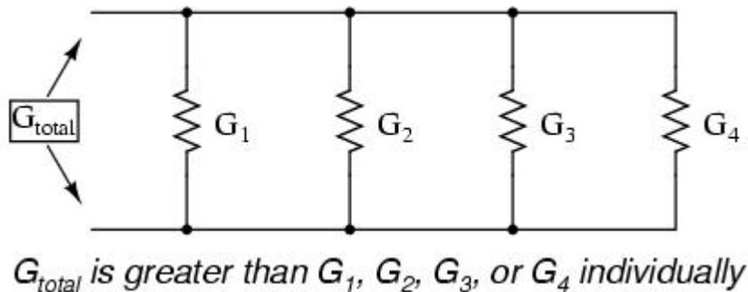
To be more precise, the total conductance in a parallel circuit is equal to the sum of the individual conductances:
