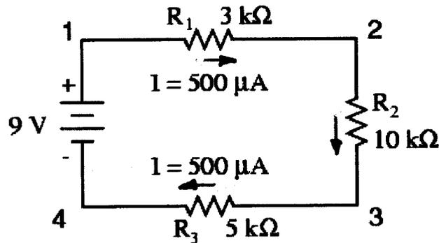
Now that we know the amount of current through each resistor, we can use Ohm's Law to determine the voltage drop across each one (applying Ohm's Law in its proper context):
