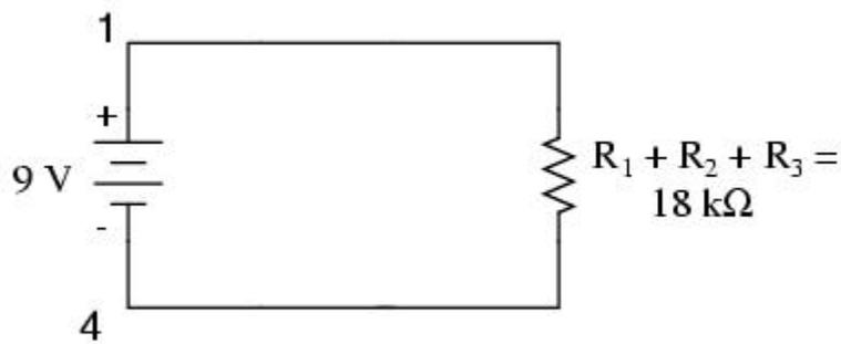
Now we have all the necessary information to calculate circuit current, because we have the voltage between points 1 and 4 (9 volts) and the resistance between points 1 and 4 (18 k $\Omega$ ):
