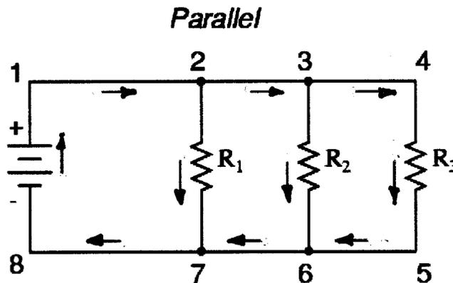
Again, we have three resistors, but this time they form more than one continuous path for current to flow. Each individual path (through  $R_1$ ,  $R_2$ , and  $R_3$ ) is called a *branch*.
