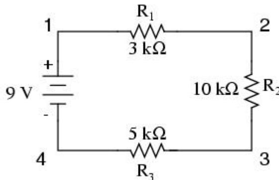
The first principle to understand about series circuits is that the amount of current is the same through any component in the circuit. This is because there is only one path for electrons to flow in a series circuit, and because free electrons flow through conductors like marbles in a tube, the rate of flow (marble speed) at any point in the circuit (tube) at any specific point in time must be equal.
