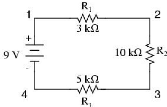
The figure of 9 volts is a *total* quantity for the whole circuit, whereas the figures of 3k, 10k, and 5k  $\Omega$  are *individual* quantities for individual resistors. If we were to plug a
