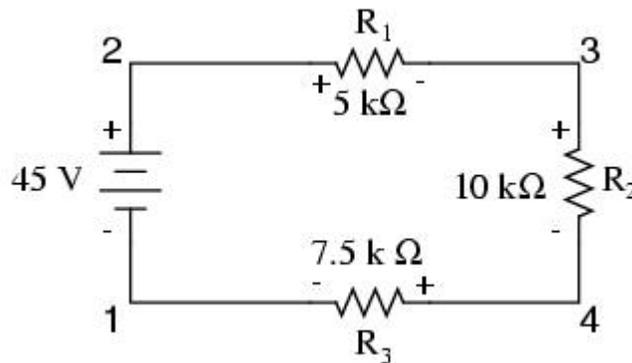
If we were to connect a voltmeter between points 1 and 2, black test lead to point 1 and red test lead to point 2, the meter would read +45 volts. Typically the "+" sign is not shown (but implied) for positive readings in digital meter displays. However, for this lesson the polarity of the voltage reading is very important:
