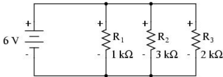
Using Ohm's Law ( $I=E/R$ ) we can calculate each branch current:
