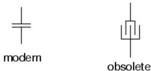
When a voltage is applied across the two plates of a capacitor, a concentrated field flux is created between them, allowing a significant difference of free electrons (a charge) to develop between the two plates:
