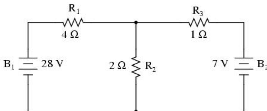
Let's suppose that we decide to designate  $R_2$  as the "load" resistor in this circuit. Thevenin's Theorem makes this easy by temporarily removing the load resistance from the original circuit and reducing what's left to an equivalent circuit composed of a single voltage source and series resistance. The load resistance can then be re-connected to this "Thevenin equivalent circuit" and calculations carried out as if the whole network were nothing but a simple series circuit:
