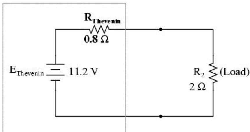
With the load resistor ( $2\ \Omega$ ) attached between the connection points, we can determine voltage across it and current through it as though the whole network were nothing more than a simple series circuit:
