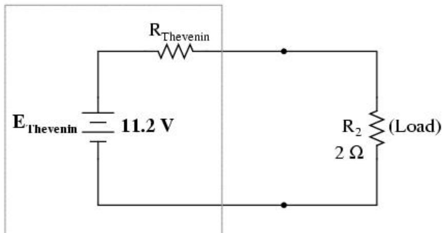
To find the Thevenin series resistance for our equivalent circuit, we need to take the original circuit (with the load resistor still removed), remove and replace by a short circuit the power sources and figure the resistance from one load terminal to the other:
