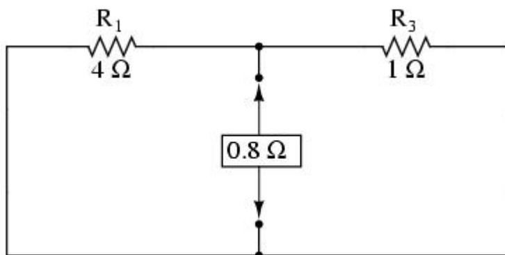
With the removal of the two batteries, the total resistance measured at this location is equal to  $R_1$  and  $R_3$  in parallel:  $0.8 \Omega$ . This is our "Thevenin resistance" ( $R_{\text{Thevenin}}$ ) for the equivalent circuit:
