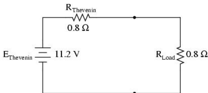
With this value of load resistance, the dissipated power will be 39.2W:
