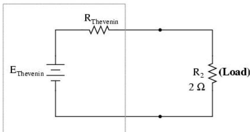
The "Thevenin Equivalent Circuit" is the electrical equivalent of  $B_1$ ,  $R_1$ ,  $R_3$ , and  $B_2$  as seen from the two points where our load resistor ( $R_2$ ) connects.
