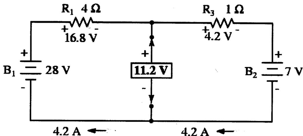
The voltage between the two load connection points can be figured from the one of the battery's voltage and one of the resistor's voltage drops, and comes out to 11.2 volts. This is our "Thevenin voltage" ( $E_{\text{Thevenin}}$ ) in the equivalent circuit:
