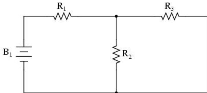
To analyse the above circuit, one would first find the equivalent of  $R_2$  and  $R_3$  in parallel, then add  $R_1$  in series to arrive at a total resistance. Then, taking the voltage of battery  $B_1$  with that total circuit resistance, the total current could be calculated through the use of Ohm's Law ( $I=E/R$ ). This current figure will then be used to calculate voltage drops in the circuit. All in all, a fairly simple procedure.
