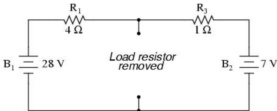
Next, the voltage between the two points where the load resistor used to be attached is determined. Use whatever analysis methods are at your disposal to do this. In this case, the original circuit with the load resistor removed is nothing more than a simple series circuit with opposing batteries, and so we can determine the voltage across the open load terminals by applying the rules of series circuits, Ohm's Law, and Kirchhoff's Voltage Law:
